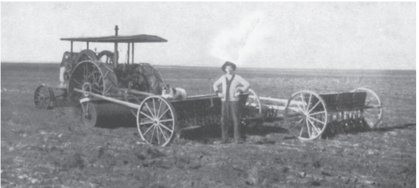
Elmer Crouch (and his bull dog) with his Case engine, the roller and then two drills seeding wheat.
