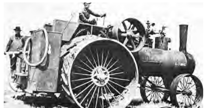
John I. Dyck at left, hired man, Jake Dyck at the controls of Case 75 - 110 steam engine with power steering, taken in 1910.
