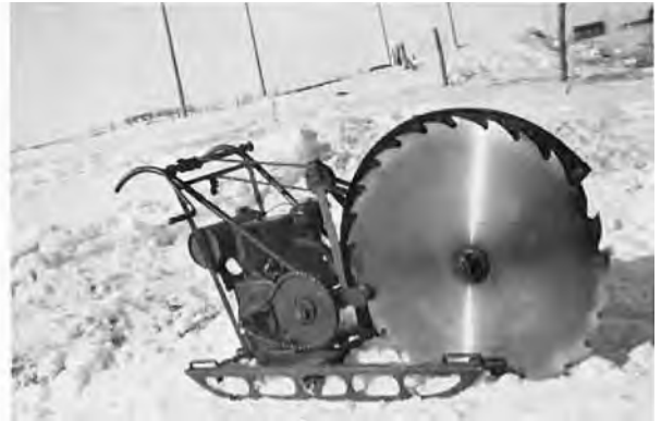
This saw was built by Dick Eidse and was extensively used to cut ice on the river in the 1940's.
