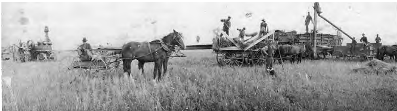
A threshing scene in the 1920's. In order to prevent fire, a 150 ft. belt was used to keep the engine back a good distance from the straw pile. A threshing gang such as this, employed 15 to 20 men. Photo courtesy P.T. Wiens.
