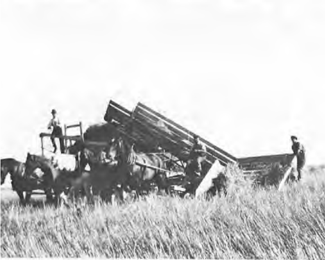
Sheaf loader on Karl Poersch's farm - used to cut the grain as well as load the sheaves.
