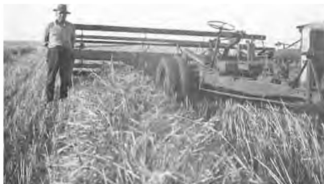
C.K. Eidse in 1944, with the self-propelled swather he built. This was one of the many useful implements he designed and built in his farm workshop.
