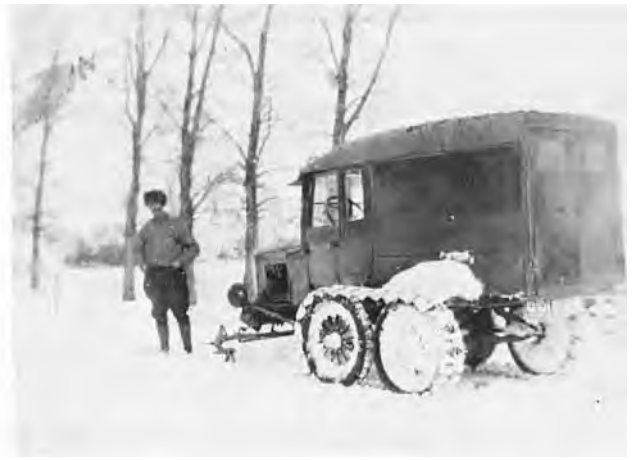
Thomas K. Bestwick (1930) probably the first mail carrier for the rural area, was a former police officer for the Town of Morris. When he retired, he hauled the mail. Someone built this all weather vehicle which had skis on the front, and track on the rear wheels. It was made to follow a sleigh track.
