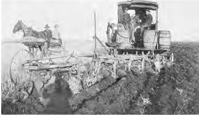
Chester Crouch's steam engine, an Undermounted Avery, doing fall plowing on the gumbo plains around Lowe Farm about 1910. Note the water barrels at rear. Photo courtesy Dan Blatz.
