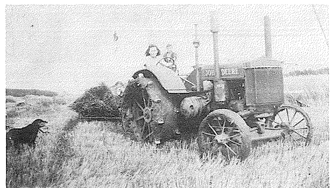
John Deere steel wheel tractor pulling a binder at Tanasychuk's farm.
