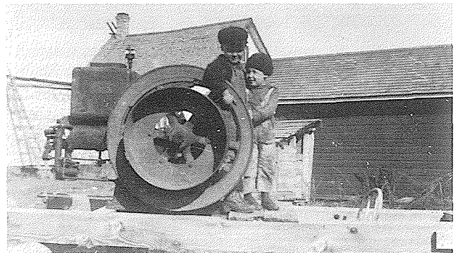
A 6-8 h.p. stationary gas engine used for sawing fire wood; used extensively in the 30's and 40's.
