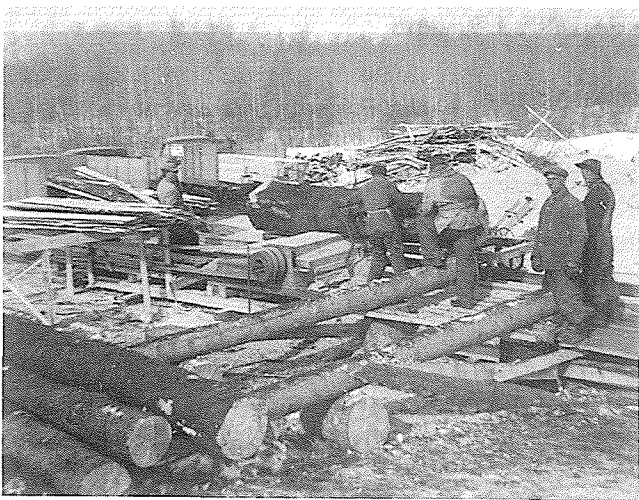
Sawmill operation on the Joe Maydaniuk Farm. Picture taken by Fred Saley shows Wm. F. Belbas (sawyer), Nestor Pushka (hooking log), and Bill H. Belbas (receiving end of log). Mike Saley and Bill H. Belbas helped to turn the huge log (40" diameter) on the carriage.
