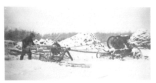
Jesse Taylor sharpening fence posts using a Hercules engine and saw.
