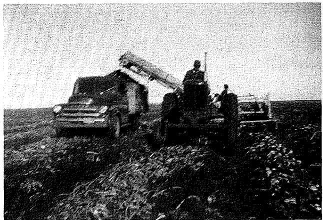
Windrows of sugar beets are loaded with a tractor-drawn loader.
